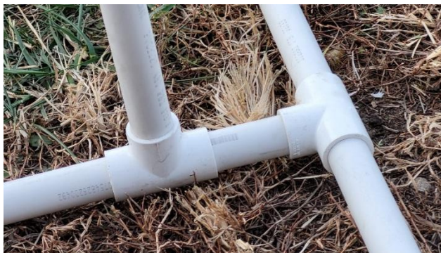
Using two \frac{3}{4} " 3-Way PVC tees to attach the support feet to the hoop
